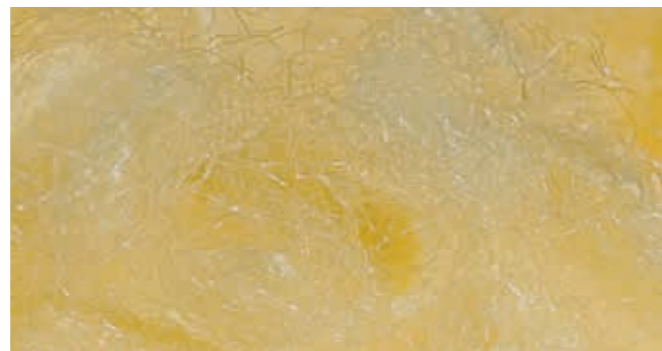
Fiber diameter: 10 microns Surface area: 1000 cm 2 /g
